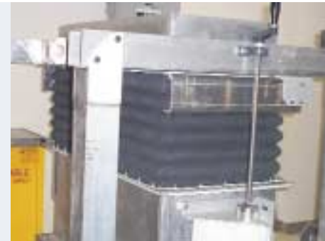
Style 1098 with 6 molded arches, Viton® tube and cover developed for Lawrence Livermore National Lab's (NIF) National Ignition Facility Program.
